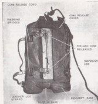
Fig. 1.—Side view of kitbag
