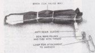
Fig. 6.—M.M.G. (C/W action) packed in Bren gun valve MR. 1
